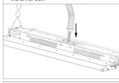
2.Insert the hook into the slotted holes as shown below.
